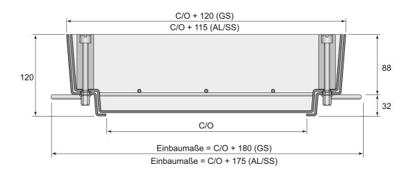
Material: Stahl verzinkt/3mm (EN 1461) ... GS\* Aluminium/3mm AlMg3 ... AL\* Edelstahl/3mm 1.4301 ... SS304\*
